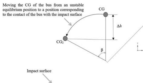
Figure 3 — Calculation scheme for determining the displacement of the CG of the bus
