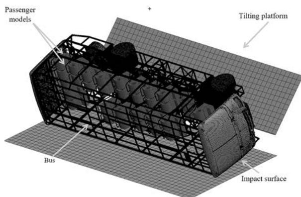
Figure 4 — Computer model for calculating the bus superstructure during passive safety tests during rollover according to the requirements of the Regulation No. 66
