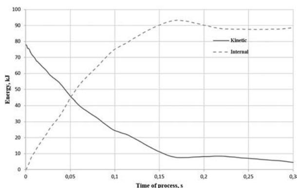
Figure 5 — Dependence diagram of kinetic and internal energy of the bus during the impact surface collision
