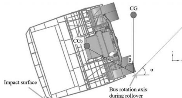
Figure 2 — Scheme for determining the tilting angles and the unstable equilibrium position of the bus
